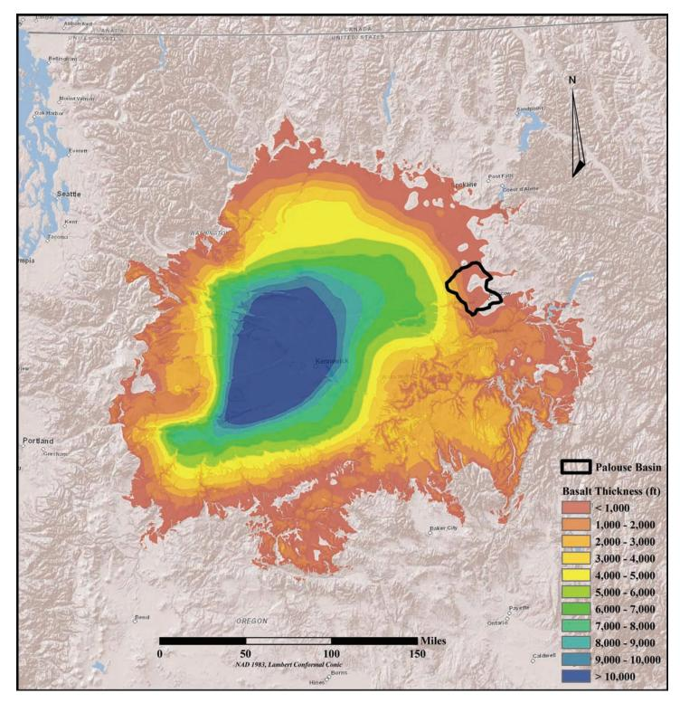
Thickness of Grande Ronde Basalt unit, Columbia Plateau Regional Aquifer System (after Burns, E.R., Morgan, D.S., Peavler, R.S., and Kahle, S.C., 2011, Three-dimensional model of the geologic framework for the Columbia Plateau Regional Aquifer System, Idaho, Oregon, and Washington: U.S. Geological Survey Scientific Investigations Report 2010-5246).
