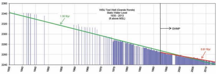
Figure 4: Static Water Level, WSU Test Well (Lower Aquifer), 1935 - 2013
