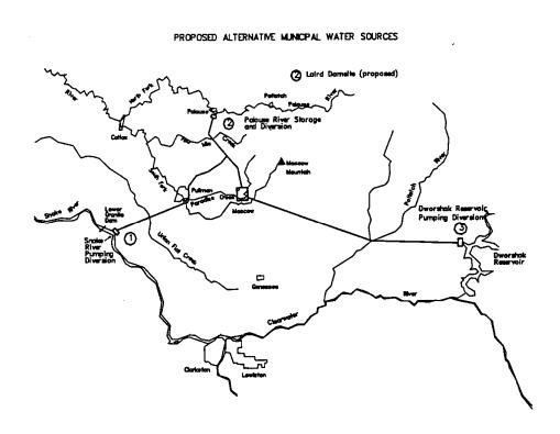
Figure 4. Proposed Municipal water Supply Alternatives (as identified by the Corps of Engineers, 1989).
