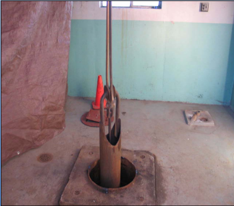
Bailer being lowered down well.
