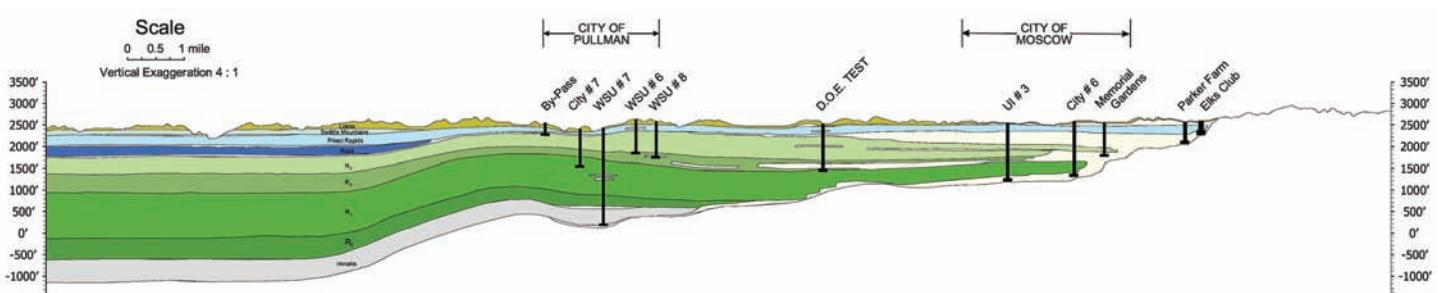
Figure 3: E-W Schematic Cross Section (Bush, Garwood, 2005)
